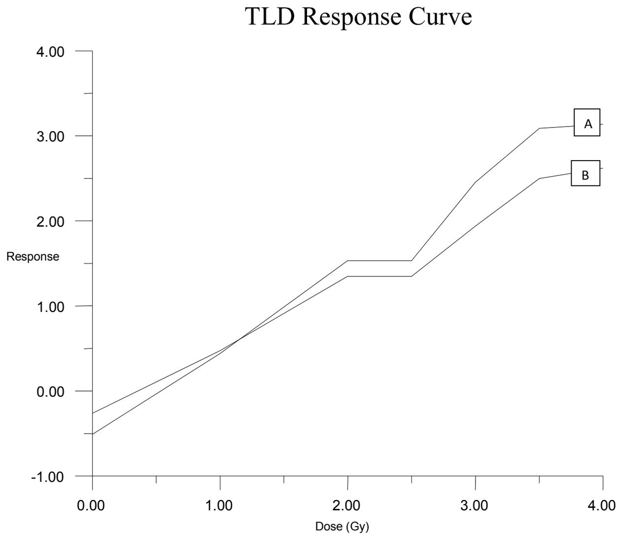
**Fig. 1: Calibration Curve for chips A and B**
