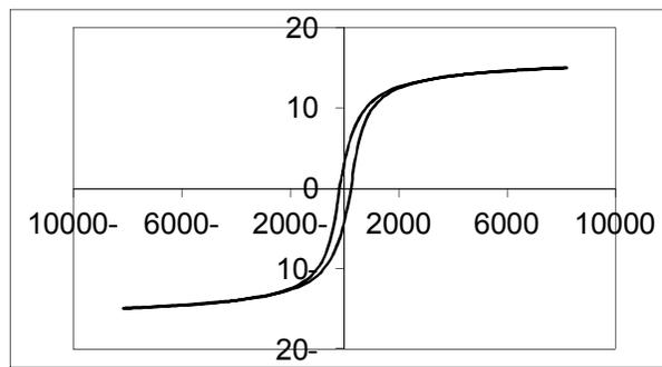
Figure 2. Magnetic hysteresis loop of NiAl<sub>0.5</sub>Fe<sub>1.5</sub>O<sub>4</sub> nanoparticles.
