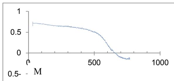
Figure 3. Curie temperature of NiAl<sub>0.5</sub>Fe<sub>1.5</sub>O<sub>4</sub> nanoparticles.
