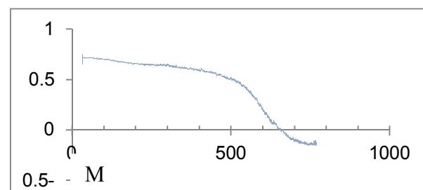
Figure 3. Curie temperature of NiAl<sub>0.5</sub>Fe<sub>1.5</sub>O<sub>4</sub> nanoparticles.
