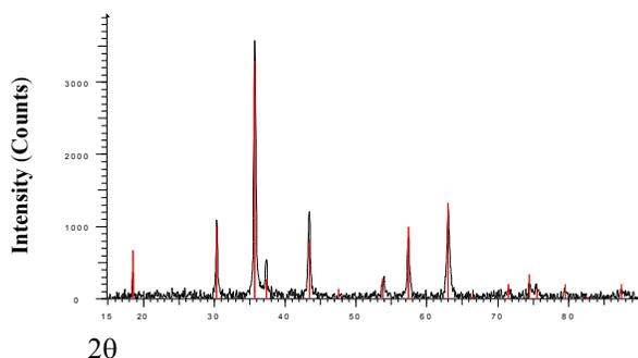
Figure 1. X-ray diffraction pattern of NiAl<sub>0.5</sub>Fe<sub>1.5</sub>O<sub>4</sub> nanoparticles.
