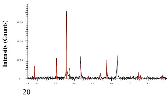
Figure 1. X-ray diffraction pattern of NiAl<sub>0.5</sub>Fe<sub>1.5</sub>O<sub>4</sub> nanoparticles.
